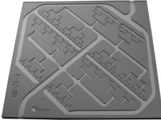
Figure 2.6 Fabricated silicon chip with dendritic channel system for cooling purposes; 40 × 40 mm footprint.
