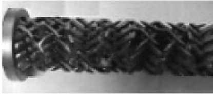
Figure 12.2 Photograph of the static mixer after premixing of the reactant fluids by a micromixer. From Ref. [8].
