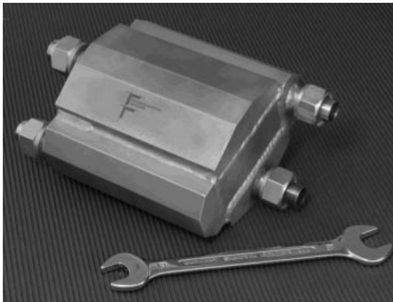
Figure 23.1 Prototype of a 5 kW reformer with integrated flue gas heating for gasoline steam reforming developed at the Forschungszentrum Karlsruhe, Germany (by courtesy of Forschungszentrum Karlsruhe).
