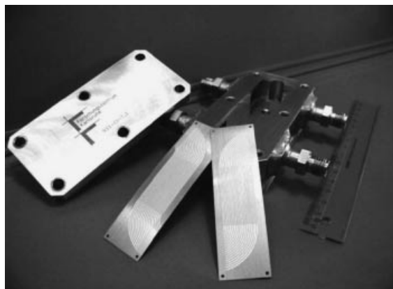
Figure 23.2 Prototype of an integrated reformer and combustor for methanol steam reforming (built at the Forschungszentrum Karlsruhe) [28].
