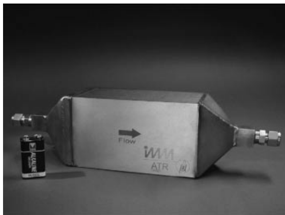
Figure 23.5 5 kW catalytic autothermal reformer built by IMM [44].
