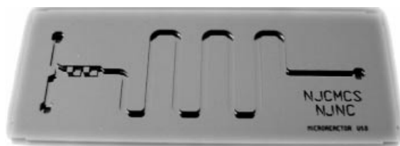
Figure 27.17 Si microchannel reactor with channel dimensions of 500 μm (width) × 610 μm (depth) × 4.5 cm (length).
