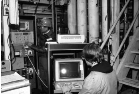
Figure 5.1 Laboratory mass spectrometer modified for data gathering in a plant environment. Courtesy Dow Chemical.
