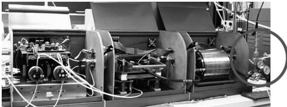
Figure 5.4 CPC continuous feed reactor with online Raman detection utilizing a commercial Raman probe equipped with a Raman ballprobe (circled) at the outlet port of the reactor.
