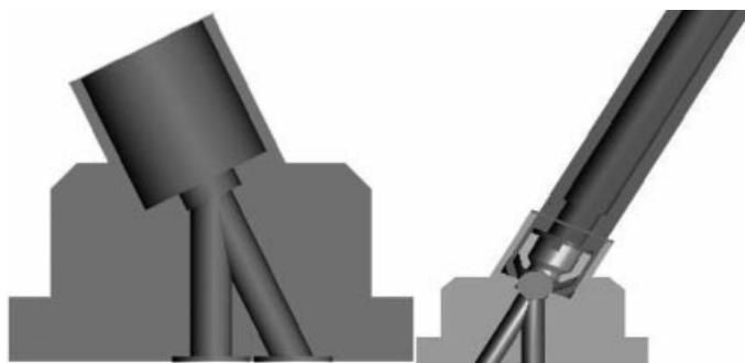
Figure 5.7 NeSSI top mount component for use with Raman ballprobe. Raman ballprobe inserted into component indicating flow channels to probe optic (sphere in right-hand illustration).
