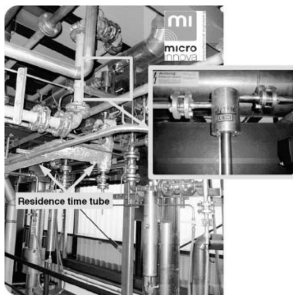
Figure 9.32 StarLam 3000 microstructured mixer retrofitted to existing plant peripherals and tank reactor (by courtesy of Wiley-VCH Verlag GmbH) [67].
