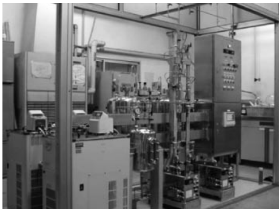
Figure 9.19 Microprocess pilot plant for Grignard exchange reaction (by courtesy of ACS) [56].
