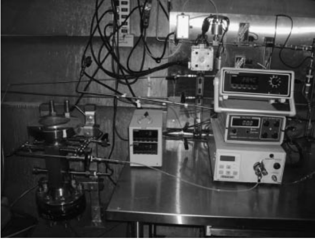
Figure 9.9 Hydrogen peroxide synthesis pilot microprocess plant by courtesy of FMC Corporation in Princeton, USA, and Niyi Lawal/Stevens Institute) [41].
