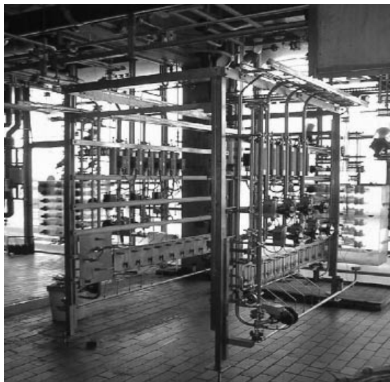
Figure 9.34 Merck production plant for Grignard-based enolate formation (by courtesy of Springer) [68].
