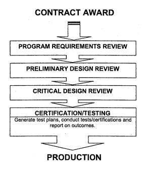
Figure 7.5 Stages in development of a product: certification/testing.
