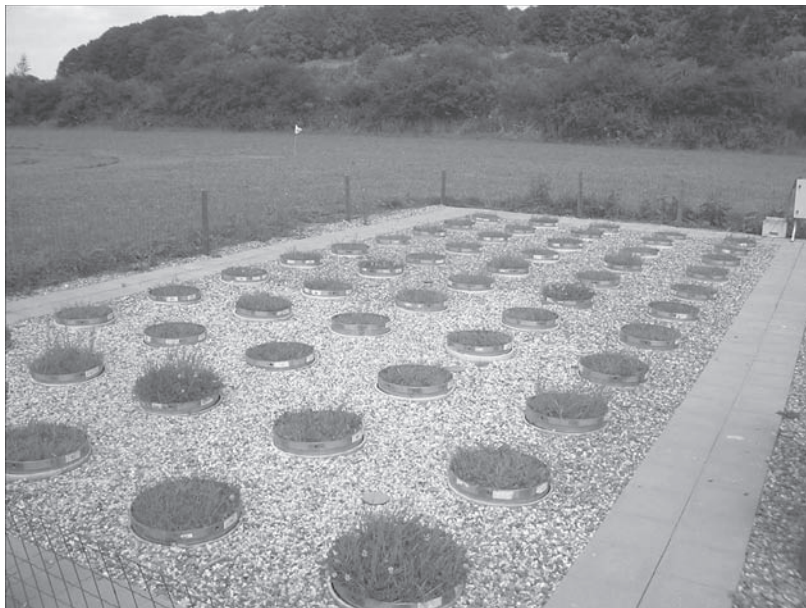
FIGURE 5.5 Outdoor experimental facility. The facility can hold up to 55 TME units that are stored on a well-drained soil-sand ground layer. (Photo by Björn Scholz-Starke.)
