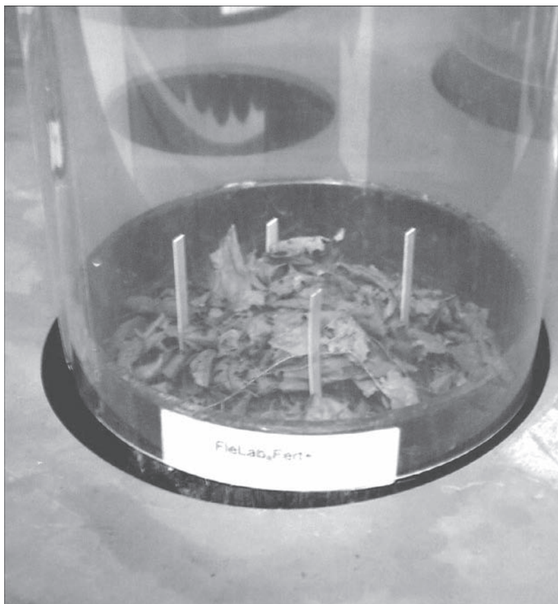
FIGURE 5.3 Conducting a bait-lamina test in a TME extracted from an agroforestry site. (Photo by Bernhard Förster.)
