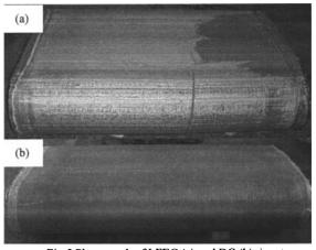
Fig.5 Photograph of LFEC (a) and DC (b) ingots
