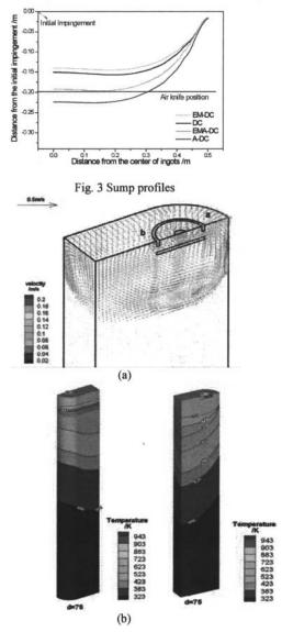
Fig. 4 Velocity vectors (a) and temperature profile (b) during EMA-DC casting process
