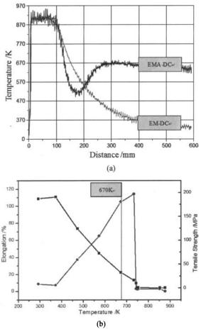
Fig. 7 The cooling curves on the ingot surface (a) and the tensile strength and elongation at the various temperature (b)
