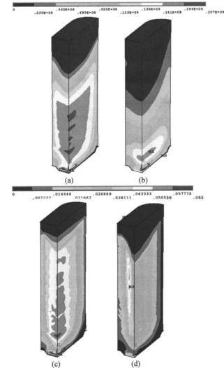
Fig. 6 Equivalent plastic stress and strain profile in the ingots in EM-DC casting (a)(c) and EMA-DC casting (b)(d) processes.
