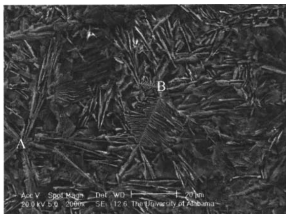
Figure 4. Longitudinal section SEM micrographs of deep etched shape cast Al-17%/Si- 3% Ba alloy, showing star-like (Points A and B) and fish bone (Point B) morphologies of silicon crystal present in the microstructure of the alloy.
