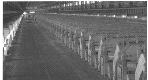
Figure 6. EMAL Phase I DX Potline.
