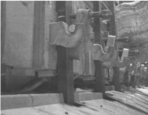
Fig. 2. Slaves mounted beneath the anode bus of the cell where the test work was done.
