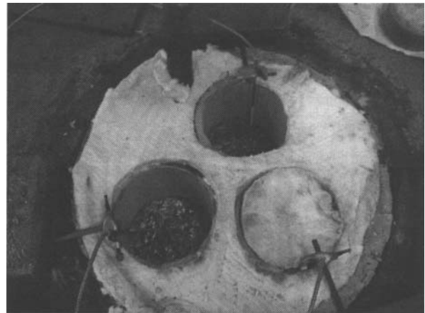
Figure 3: Three crucibles with molten aluminium from uncoated and coated sheets placed inside a resistance furnace to ensure otherwise equal conditions.
