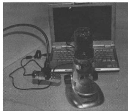
Figure 1. Baked anode optical macroscopy arrangement using a USB microscope (Traveler model number SU 1071). Note the oblique lighting to shadow surface porosity. As long as it provides
