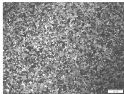
Figure 2 – As received ZEK100 feed stock material that was symmetrically rolled to the starting gauge of 2.18mm for asymmetric rolling.
