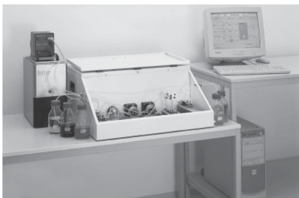
Figure 1.10 Hybrid, multi-scale micro-reactor plant, a commercial product of mgt mikroglas technik AG, Mainz, Germany [9].
