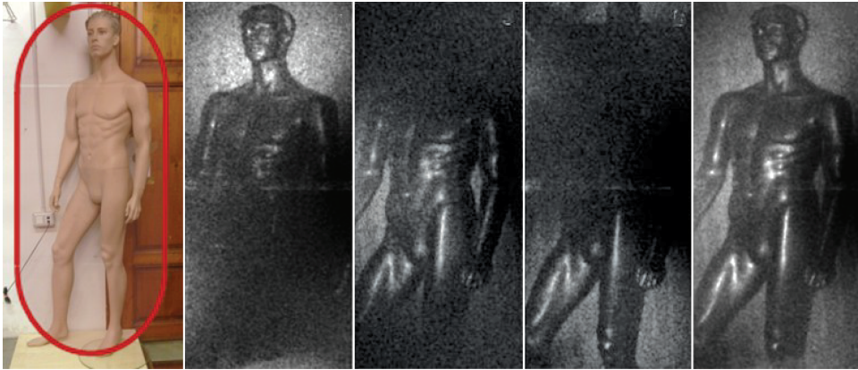
Figure 2.10 (Plate 4) (From left to right) Mannequin image with irradiated area in red; mannequin hologram amplitude reconstruction at different scanning time and superposition of the most significant frames. See plate section for the color version
