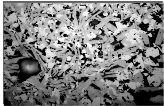
Figure 4. Microstructure of sinter with 5 % LARM. Residual grains of magnetite– white, ferrite – grey, glass phase – dark grey. Reflected light, magnification \times 500 .
