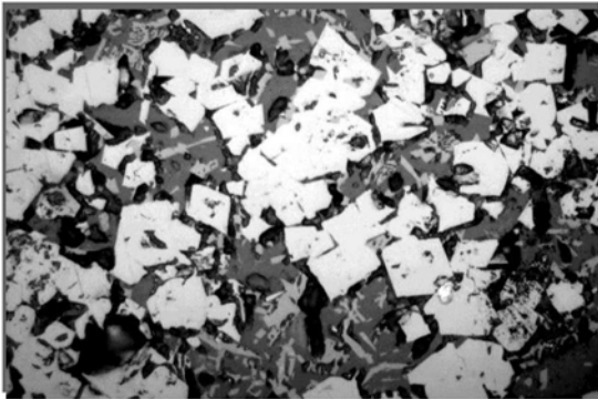
Figure 2. Microstructure of sinter with 1 % LARM. Glass phase – grey, needle crystals of ferrite – light grey. Reflected light, magnification \times 500
