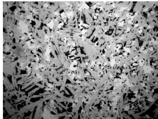
Figure 5. Microstructure of sinter with 7 % LARM. Residual grains of magnetite– white, ferrite – grey, glass phase – dark grey. Reflected light, magnification \times 500 .
