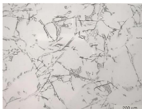
Figure 4. Microstructure of H1 alloy sample obtained at 100mm level above the chill end showing the relative abundance of \beta\text{-Al}_3\text{FeSi} needles.
