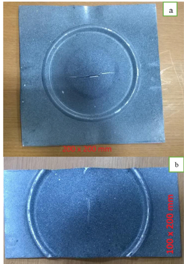
Figure 4. Deformed sample (a) sample of 200x200 mm 2 deformed SM; (b) A sample of 200x100 mm 2 deformed SM
