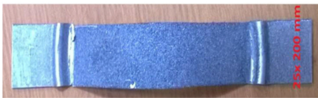
Figure 3. Fracture of reduced-width rectangular specimen during the test
