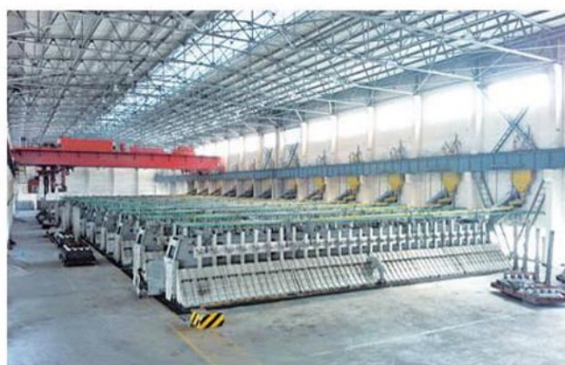
Figure 1. 600 kA pot in the pilot plant [3]
