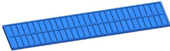
Figure 2. The geometry domain for two phase flow of aluminum reduction pot
