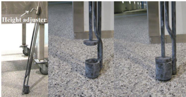
Figure 1. Sampling device used for taking samples during power outage
