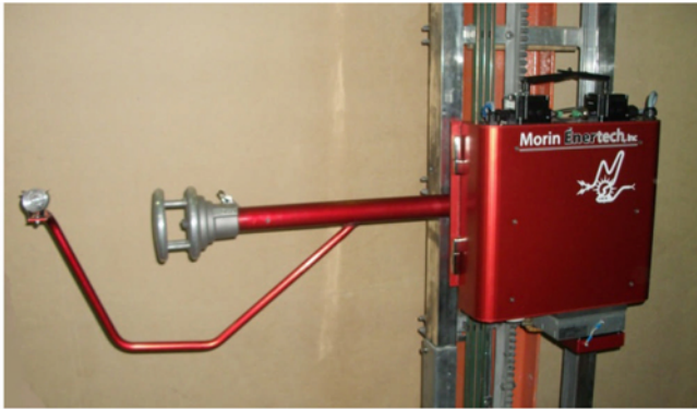
Figure 2: The mobile SHERPA box on its rail
