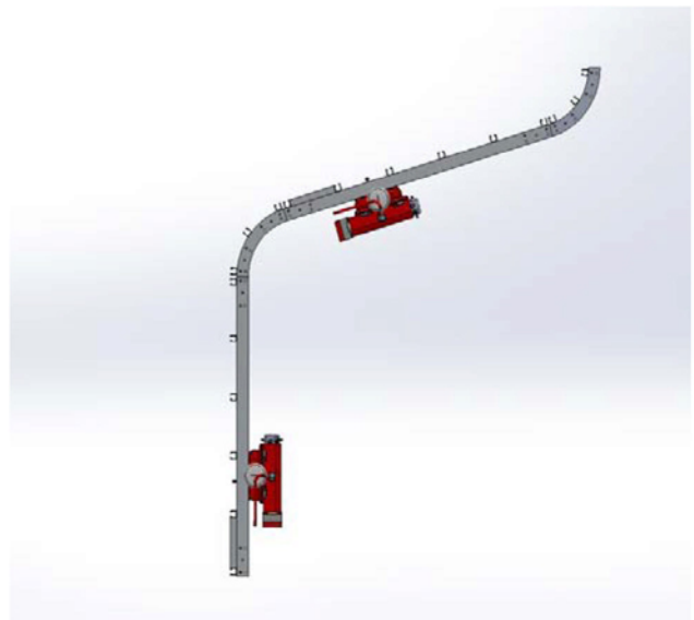
Figure 5: The mobile shuttle can take different positions along the rail.
