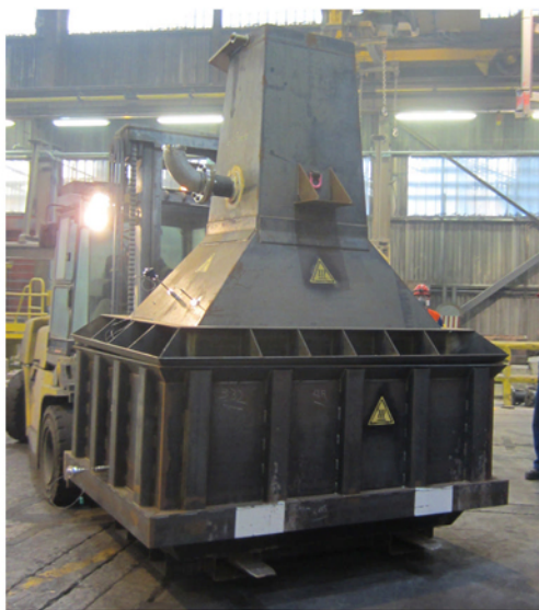
Figure 2 – Prototype of new anode cover concept
