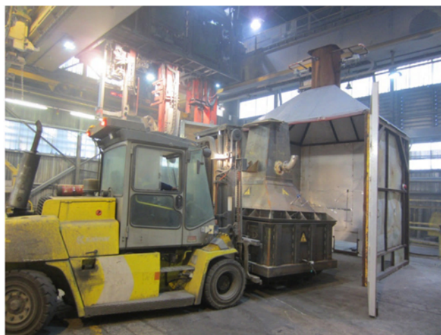
Figure 3 – Covered spent anode being introduced into the measurement enclosure
