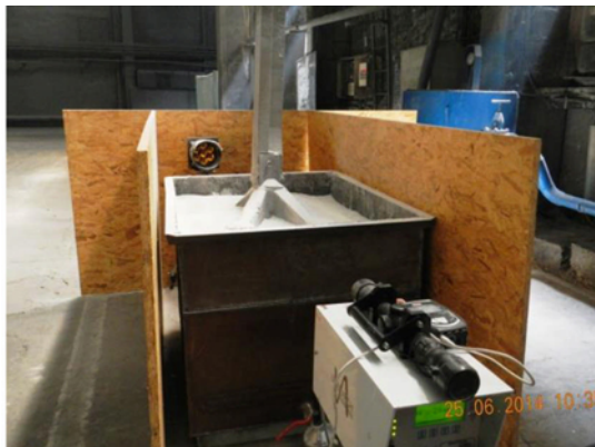
Figure 6. HF measurement on spent anode buried in alumina
