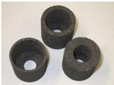
Figure 6. Anode carbon samples with 40 mm external diameter and 2.5 mm, 5 mm, and 10 mm wall thicknesses.
