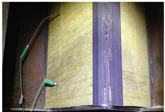
Figure 4. An example of potshell insulation on a pot corner
