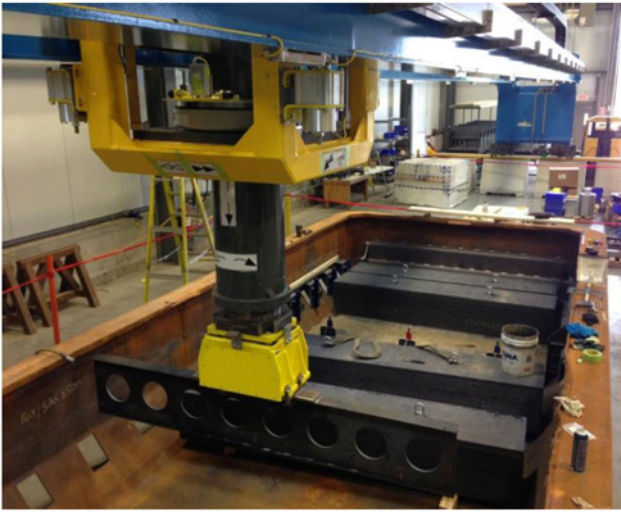
Figure 9. Full scale bench test with a P155 shell in the shop
