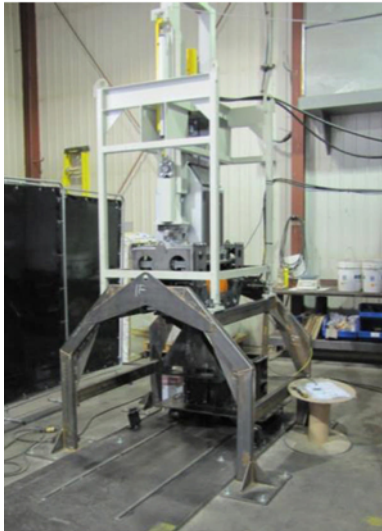
Figure 1. Full scale compaction bench test.
