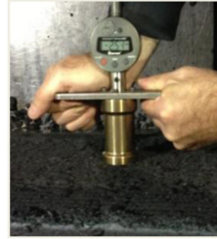
Figure 4. Custom-made hardness measuring instrument, commonly known as a penetrometer, used mainly to compare different compaction works and check compaction homogeneity through a layer.
