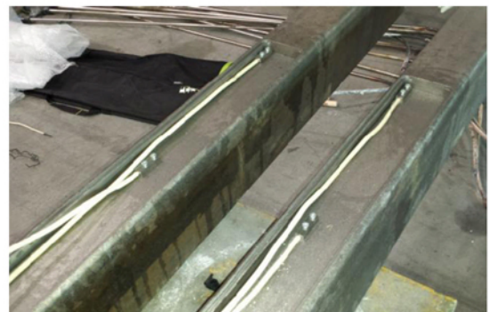
Fig 17: In-situ measurements of temperature and electric potential
