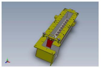
The distribution launder has a gate at one end to empty its content into a pan in case of an emergency stop.
