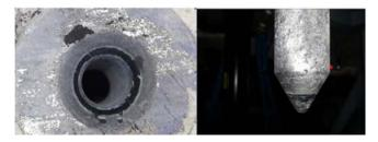
The spout diameter is set according to the desired metal flow. The spouts are made of individual cast parts inserted in the bottom of the launder refractory. Metal flow is calculated based on the time available to fill the moulds.
