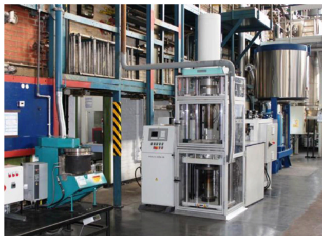
Figure 1: Pilot anode facility showing IR heated Eirich mixer, hydraulic press and baking furnace
