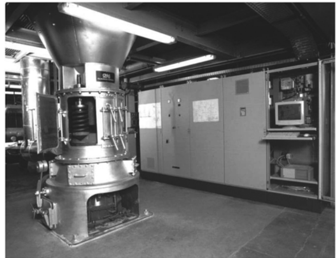
Figure 4: EM 17-525 Test Mill with Control System
