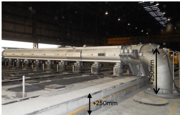
Figure 13: Exhaust manifold with modified vertical section
