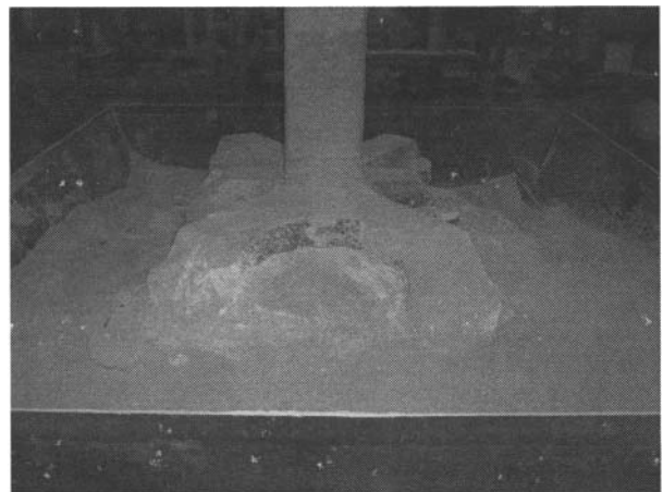
Figure 9 - Spent anode covered with cover mix
