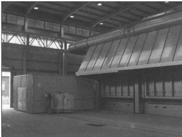
Figure 6: Twin chamber furnace with docking type charging machine
