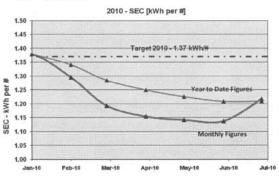
The blue dashed line is the target for the year of 1.37kWh/#. The red line reports monthly SEC and the green reports the Year to Date Figure. It can be seen that the performance is better than target.
