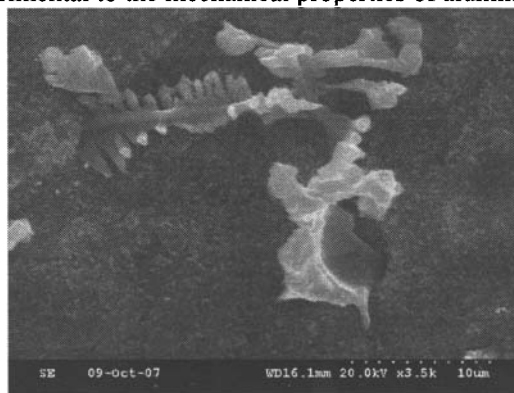
Figure 1. 3-D morphologies of Fe-rich intermetallic phases of \beta -Al(FeMn) 3 Si [5].
