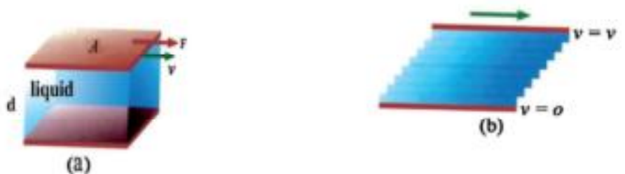
Force acting on the upper layer of a liquid
