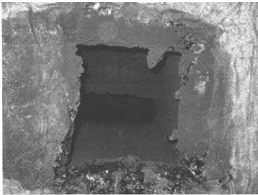
Figure 5: Bottom view of a flexible exhaust boot (97% pitch burn)
