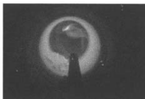
Fig. 14. Undesired shape of flame obtained upon calcination of coke Y in BP lab kiln
