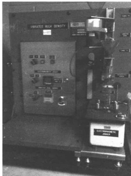
Figure 3: STAS' semi-automated VBD apparatus. Photo courtesy of Rain CII Carbon, LLC.
