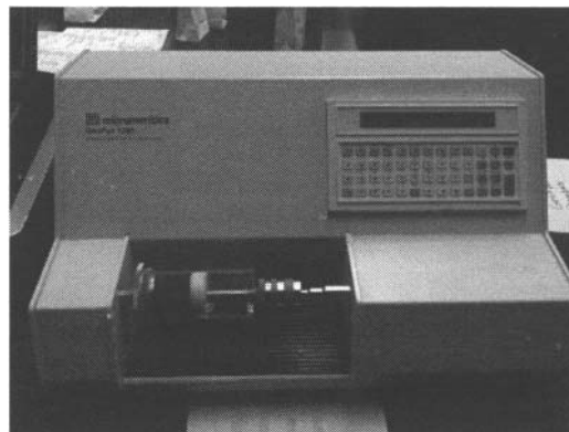
Figure 4: GeoPyc apparatus (Micromeritics model 1360). Photo courtesy of Rain CII Carbon, LLC.
