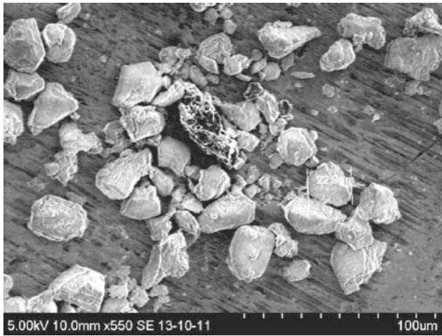
Figure 8 SEM picture of the secondary alumina fine sample № 2 ( D_{50} = 20 \mu\text{m} ).
