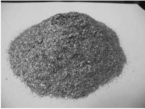
Fig. 14. Ribbons cast from AlSi30Cu1.5Mg1.2Ni1.5Fe0.8 alloy fragmented to the form of chips.
