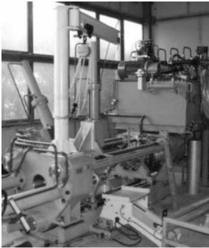
Fig. 2. A horizontal direct-indirect press of maximum 500T capacity.
