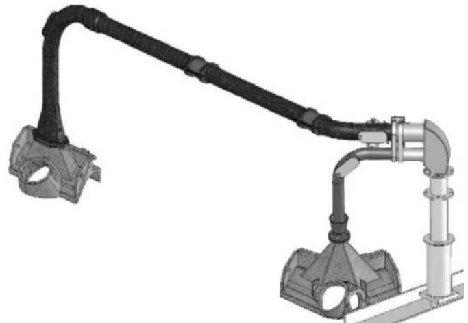
Figure 3. 4-dome gas collection system (one side)
