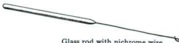
Glass rod with nichrome wire (for flame testing)
