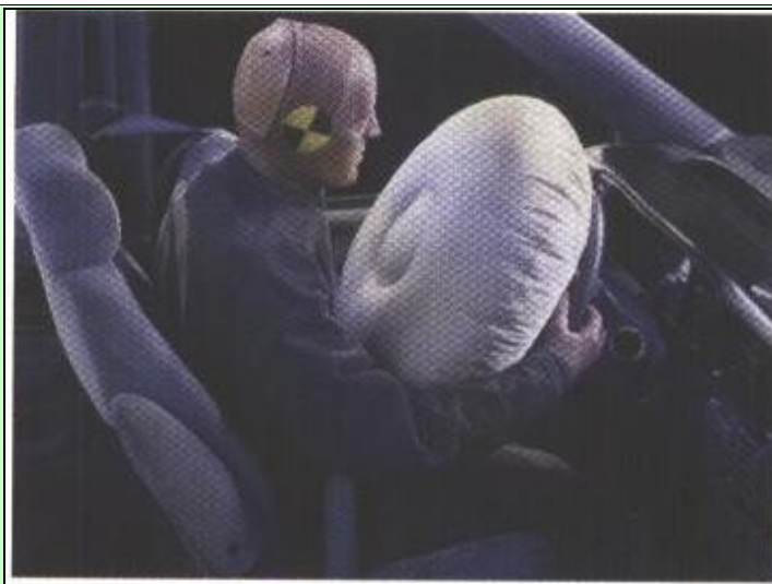
Fig. 55 : Automobile air bags are inflated with N_2 gas produced by decomposition of sodium azide
