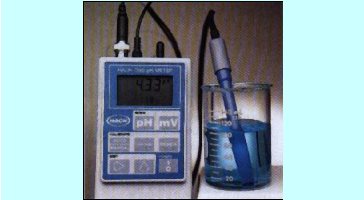
Fig. 72 : A pH meter uses the voltage of a cell to measure the H^+ concentration in a solution. Each change of one pH unit causes a voltage change of 0.0592 volts.
