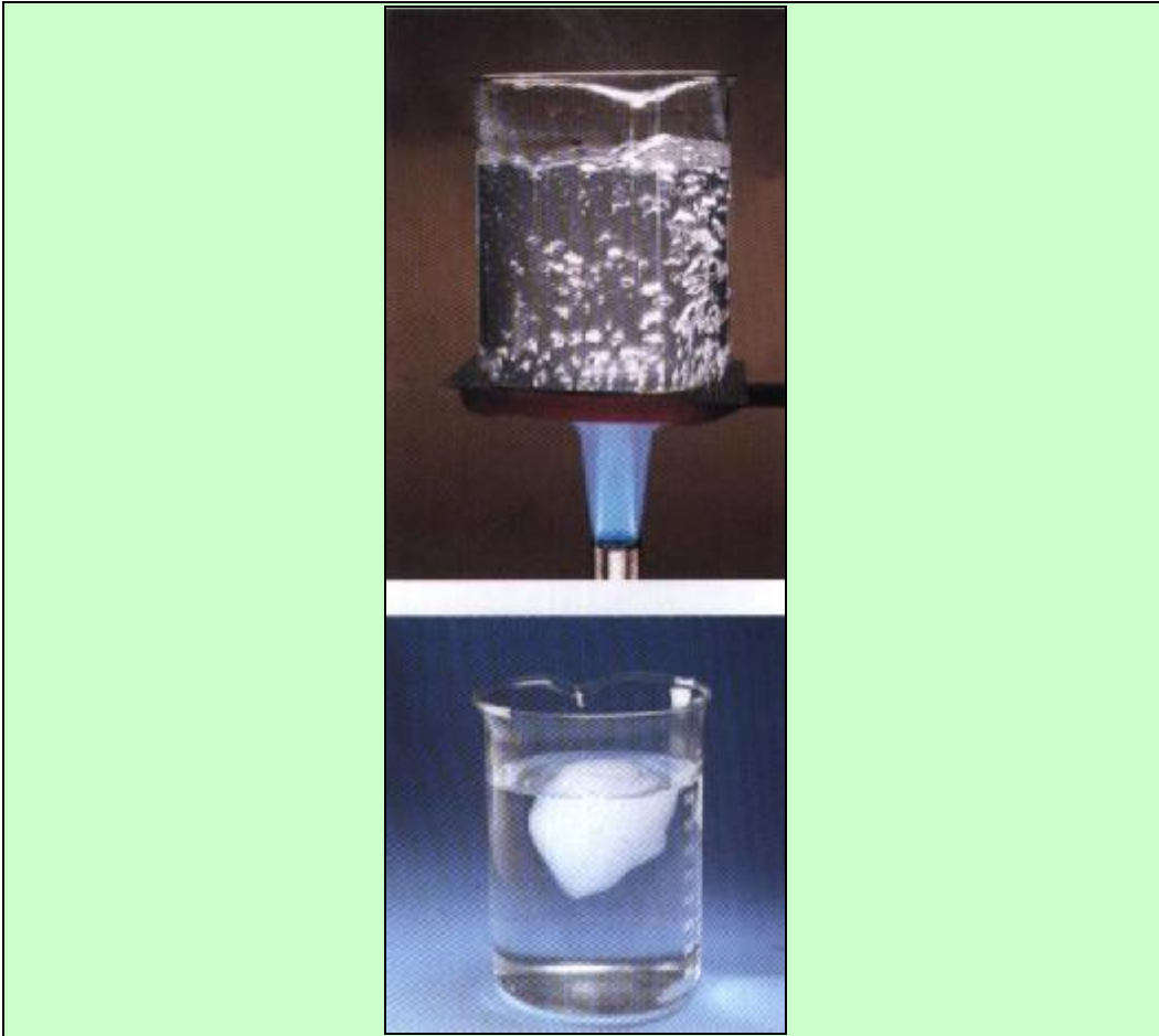
Fig. 50 : During any phase change, liquid \rightleftharpoons gas and solid \rightleftharpoons liquid the temperature remains constant.
