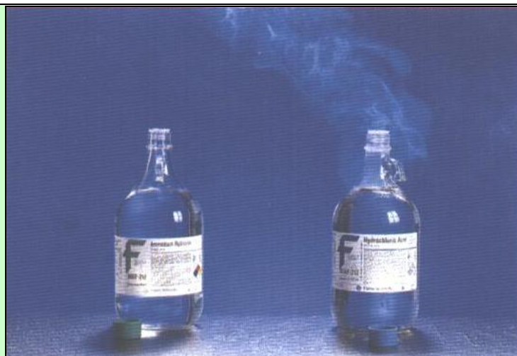
Fig. 87 : A demonstration of gas diffusion. \text{NH}_3 gas (from a bottle containing aqueous ammonia) combines with \text{HCl} gas (from a bottle containing hydrochloric acid) to form solid \text{NH}_4\text{Cl} . Because \text{NH}_3 is lighter and therefore diffuses faster, solid \text{NH}_4\text{Cl} first appears neared the \text{HCl} bottle (on the right).
