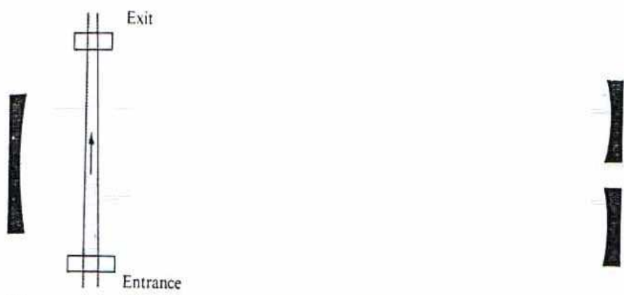
(A) 10-cm path (plane mirror retracted)
