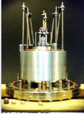
( Fig.1.6 ) Scanning tunneling microscope , with eddy current damping developed in our group. [12]
