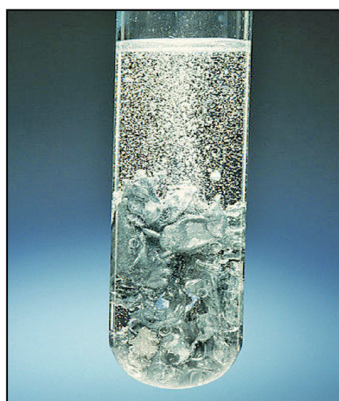
Reaction of zinc with HCl
